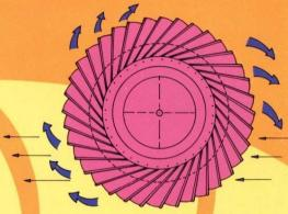
breeze will cause the turbine to spin and even after the breeze has stopped, the fly wheel effect of the rotor cage will use its stored energy to continuously remove air giving rise to ventilation. Suction is maintained even at low wind velocities.
